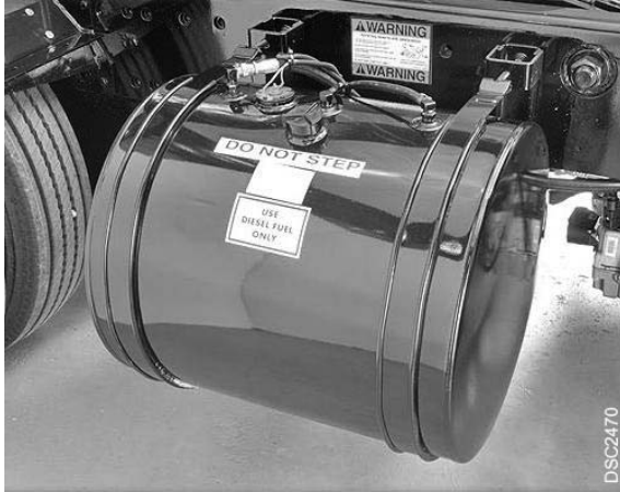
Fuel Tank and Fittings
