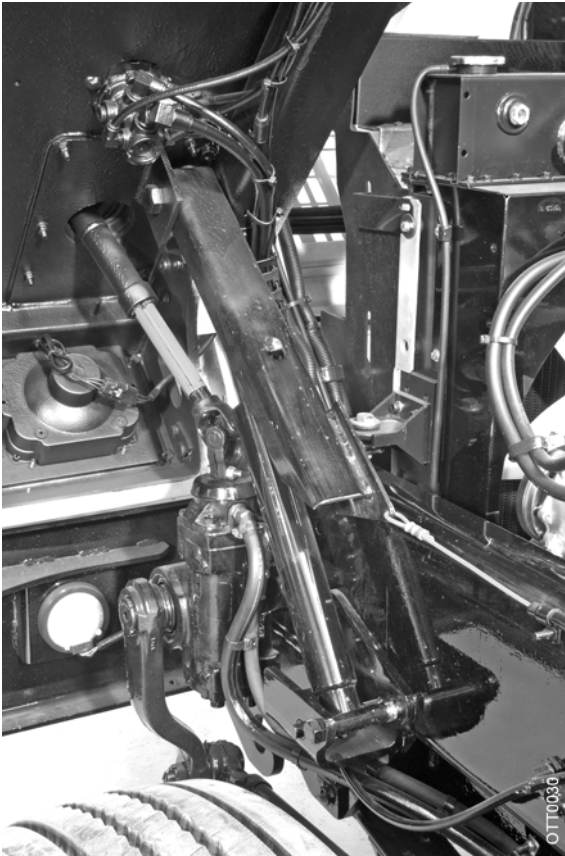
Cab Tilt Cylinder and Safety Prop
